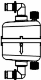
2QE 1/4" Male quick coupling, elbow
