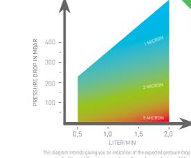
ints plagram intends giving you an indication of the expected pressure grop over the filter at different micron ratings. Depending on the type of filter media used (eg Polypropylene or Glass Fiber), the pressure drops can differ substantially, therefore the large scatter on the diagram.
